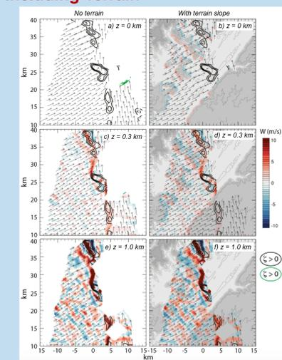
Dual-Doppler wind syntheses (horizontal winds are vectors, vertical velocity is shaded) at various levels above the bottom of the grid (at z = 0, 300, 1000m) that assume: flat ground at z = 0 km (left) and sloped terrain (right). Fields are overlaid on top of USGS topography (gray shaded).
